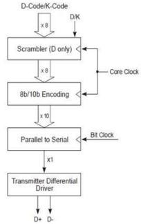
Figure 4 Transmitter Block diagram
