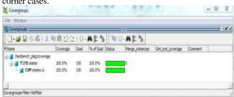
Figure 9 Functional coverage for state transitions for LTSSM
