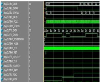
Figure 10 PHY layer interface waveform
