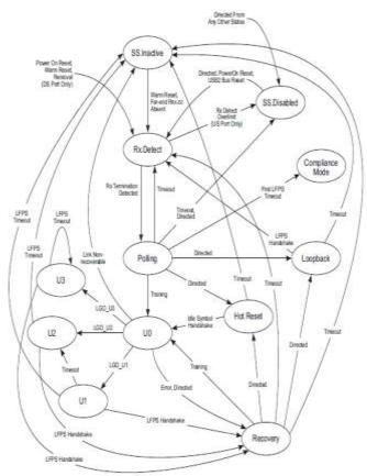
Figure 6 State Diagram of the Link Training and Status State Machine
