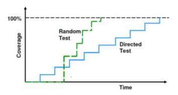
Figure.1. Random test Vs Directed test
