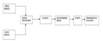
Fig 1(b):Block diagram for Affine Transform
