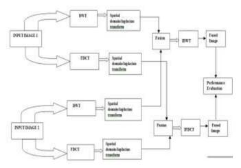
Fig 1(a):Block Diagram for Multilevel Fusion Method
