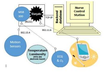
Fig 5: Monitoring system at Nurse Control station.
