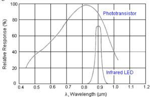
Fig: Response of phototransistor and Infrared LED
