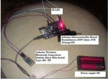
Fig.: Bluetooth Module interface with ATmega 328 development board
