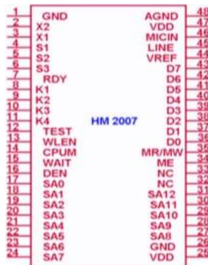
Figure 2. Functional Pin Description of HM2007
