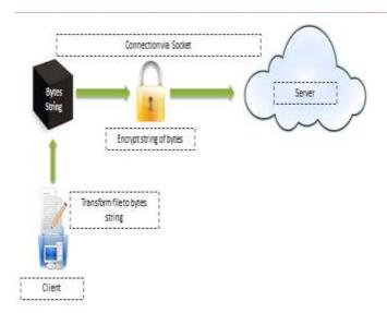
Fig. 1 Sending data from the customer to the server program
