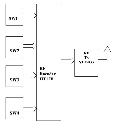
Fig1: Transmitter Module
