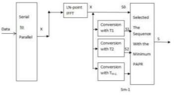
Figure 2 Modified SLM
