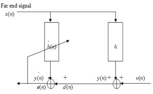
Fig.1 Function diagram for system identification
