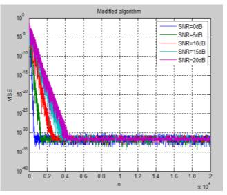
Fig. 4 Comparison of the OVSS-NLMS with conventional approach with different MSE
