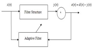
Fig.1 Block Daigram for system identification
