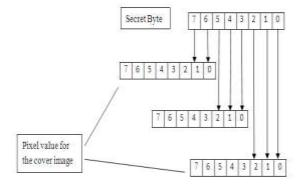
Fig.3.6: Concealing mechanism inside steganography block
