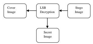
Fig 3.3: Block diagram of decryption of an image.
