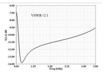
Figure 4. S-Parameter v/s Frequency of Main Antenna.
