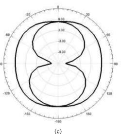
Figure 6. Radiation plots of (a) Main Antenna at 1 GHz (b) Main Antenna at 1.5GHz (c) Subsidiary Antenna at 2.5 GHz.
