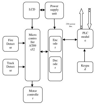
Figure 2. Block Diagram of Receiver Section
