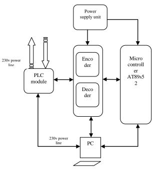
Figure 1. Block Diagram of Transmitter section
