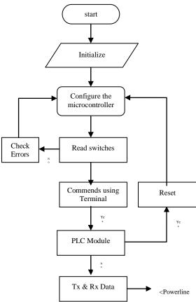
Figure 4. Flow Chart for Transmission Section
