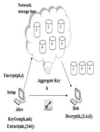
Fig 2 usage KAC for data sharing in cloud storage In order to share the data to the cloud the Alice (sender) will first perform the setup in order to have an public system
