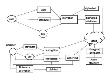
Fig 3 the general architecture of usage of cryptography in cloud
