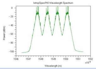
Fig. 6 multiplexed upstream data signal at the output of wdm mux 2
