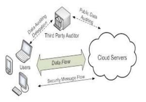
Figure 1. The architecture of cloud data storage service
