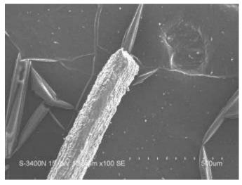
Fig.2 SEM image of fractured fiber after tensile test Fig.2 and Fig.3 shows the SEM image of fractured fiber after tensile test and flexural test respectively. It is shows modification in the surface of the fiber, which is increase the binding capacity with the resin. Surface roughness is increase the strength of the material. During the tensile and flexural test, the fiber comes out from the matrix. It is visible in SEM image.
