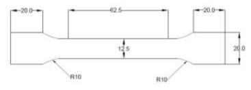
Fig.1 Dimensions of tensile test specimen
