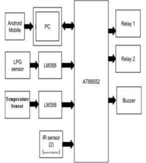
Figure1: Block Diagram
