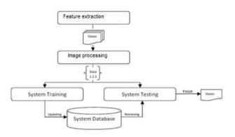
Figure 1: Architecture of Gesture recognition system
