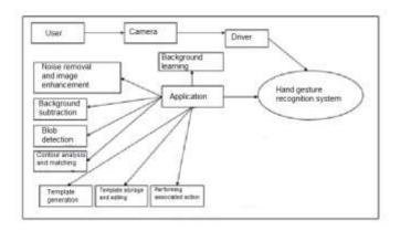
Figure 3: Data flow diagram of the system
