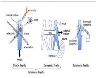
Fig. 1.Physical traits used by motion sensors.
