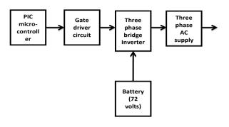
Figure:-1 Block diagram of Hardware implemented system
