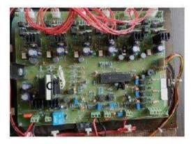
Figure: -4 Photographic view of three phase Inverter circuitry
