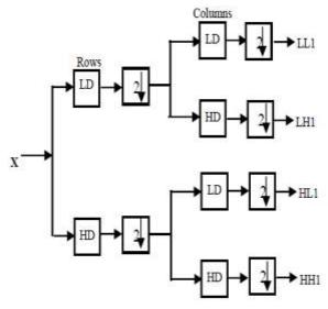
Figure .1 Wavelet filter bank of one level image-decomposition
