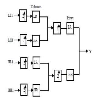
Figure 2 Wavelet filter bank of one level image-Reconstruction IV. Shrinkage Techniques
