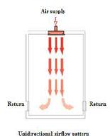
A cleanroom requires a very stringent control of temperature, relative humidity, particle counts in various rooms, air flow
