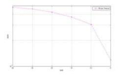
Figure 3 BER: QAM over RICIAN channel
