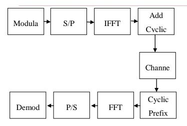
Figure 1.1: OFDM trans-receiver
