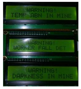
Figure 7 Miner's Module Alert System
