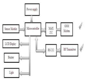
Figure 2 Block Diagram of the miner module
