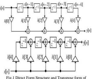
Fig.1 Direct Form Structure and Transpose form of direct structure
