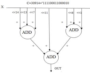
Fig .3.Graph Based Algorithm
