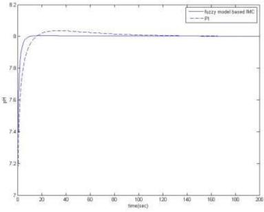
Fig 7. Servo response for pH change from pH 7 to pH 8
