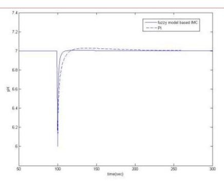
Fig 12. Regulatory response for disturbance of -1 pH
