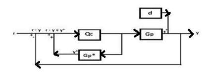
Fig 3. Block diagram of IMC based PI controller
