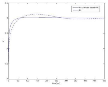
Fig 8. Servo response for pH change from pH 7 to pH 9
