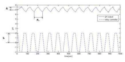
Fig 5. Relay feedback test for pH process
