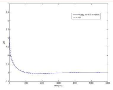
Fig 10. Servo response for pH change from pH 7 to pH 3
