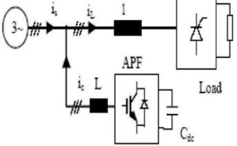
Figure1: Basic system with Non-Linear Load and Shunt Active Filter
