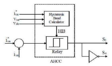
The current and voltage waveform for phase 'a' is shown here where Isa\* is the desired reference source current and Isa is the actual source current. When the source current tries to leave the hysteresis band appropriate switch is turned ON or OFF to force the ramping of the current within the hysteresis band.
