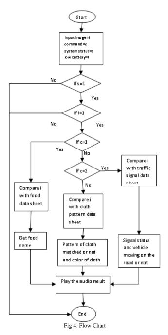
Start the program, let we consider the input image is i, and speech command is consider c, and the system status for on or off condition is consider s, and low battery level is consider s. If the system is on s=1, if the condition is yes go to next stage and the system is off the condition s is not equal to s go to end. If the low battery level is s l=1 go to end and s is higher level go to next stage.[3] If the command is s level go to food identification images
