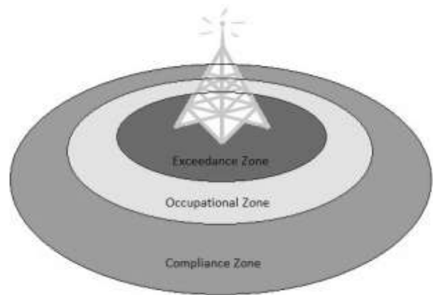
Figure 3. Different zones around the Base Transceiver antenna
