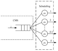
Fig.2.Scheduling subsystem model
