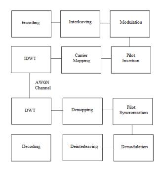
Figure 2. Wavelet based proposed OFDM system design.
