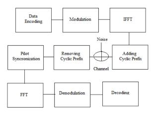
Figure 1 DFT based OFDM transmitter and receiver
