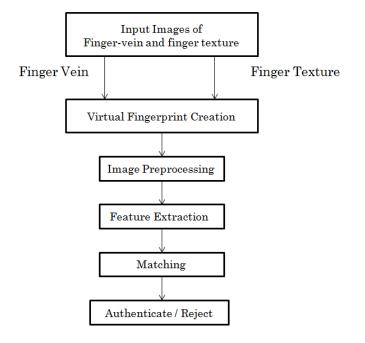
Fig. 1. Block Diagram for the proposed personal identification using finger-vein and finger texture combination
