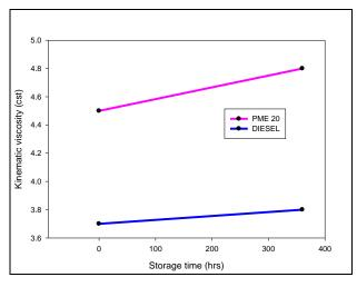
Figure 6: Viscosity vs. storage time at 40 °C.
