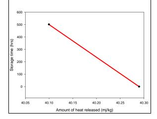
Figure 1: Comparison of the heat release of palm-oil biodiesel at various storage temperatures and times
