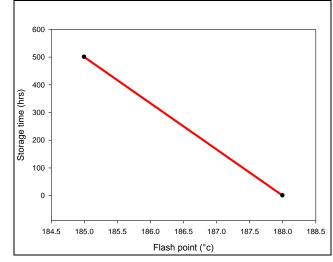
Figure 3: Comparison of the flash point of palm-oil biodiesel at various storage temperatures and times
