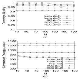
Figure 2. Performance analysis a. Coverage quality b. Energy Consumption
