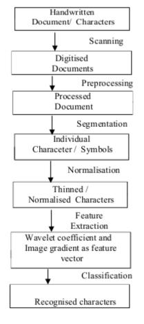
Fig. 2. Block diagram of proposed solution.
