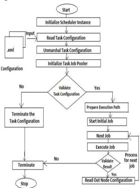
Fig. 5: Flow Diagram of Cyclic Job Scheduling Algorithm
