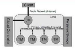
Fig. 2: Basic Design Architecture of Nephele Framework [1]
