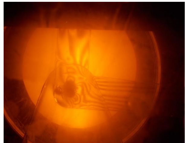
Figure18. Isochromatic fringe pattern developed in photoelastic model of bell crank lever
