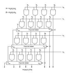
Figure 5: Braun Array Multiplier
