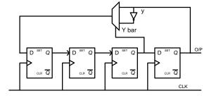
Figure 3. MUX based LFSR B. Bit Flipping LFSR
