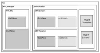
Figure 8: Top component and hierarchy of other components that are inside it.
