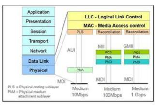
Figure 2: The OSI and generic Ethernet Physical Layer model
