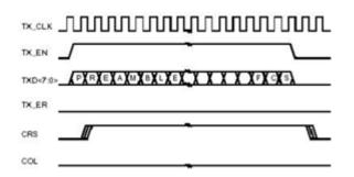
Figure 5: GMII Transmission timing for packet with no error
