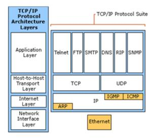
Figure 3: Top protocols and networks in the TCP/IP model
