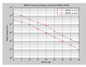
Figure 8 . MSE for MMSE estimation of 2x2 and 4x4 MIMO-OFDM system
