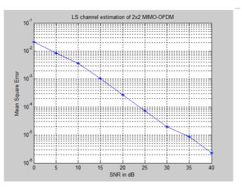
Figure3. MSE for LS estimation of 2x2 MIMO-OFDM system
