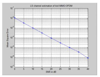
Figure 5. MSE for LS estimation of 4x4 MIMO-OFDM system
