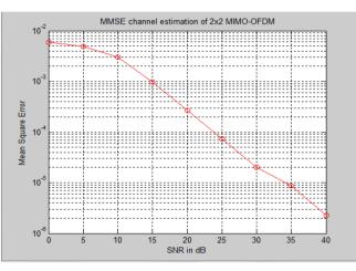
Figure 4 . MSE for MMSE estimation of 2x2 MIMO-OFDM system
