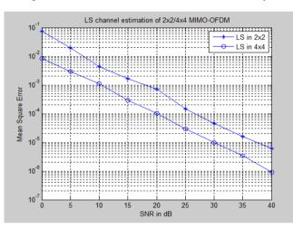
Figure 7 . MSE for LS estimation of 2x2 and 4x4 MIMO-OFDM system
