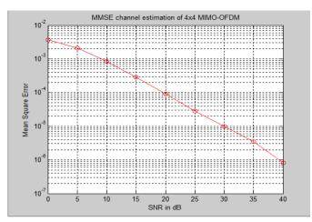
Figure 6 . MSE for MMSE estimation of 4x4 MIMO-OFDM system
