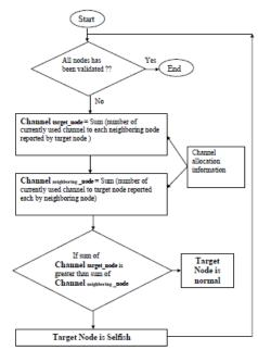
Fig 5 Algorithm for Detection Mechanism
