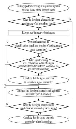
Fig. 1. A flowchart of the transmitter verification scheme
