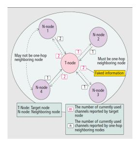
Figure 4. Selfish attack detection mechanism
