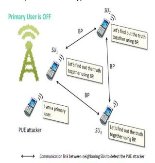
Fig: 2. Illustration of belief propagation based detection against PUE attack in cognitive radio networks
