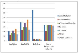
Figure 7. Comparison parameters of different multipliers.
