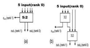
Figure 4. Wallace tree multiplier using 5:2 compressors
