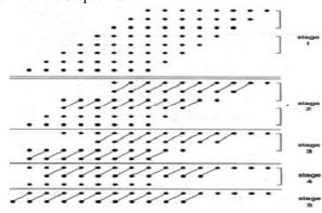
Figure 2. Wallace tree internal structure.
