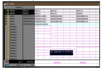
Figure 6. Simulation output waveform of Dadda.
