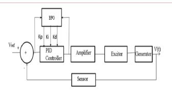
Fig.2: The Block Diagram of BFO algorithm based PID controller.
