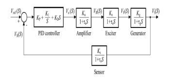
Fig.1: Block Diagram of AVR System with PID Controller.
