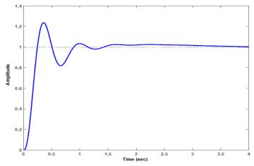
Fig.4: Step response of AVR system with PID controller using Ziegler-Nichols tuning method
