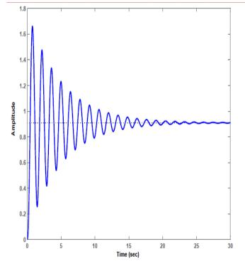
Fig.3: Step Response of AVR System without PID Controller
