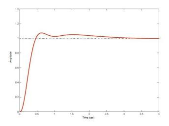
Fig.5 Step response of AVR system with PID controller using BFO tuning method
