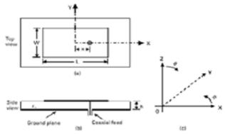
Figure 1. (a) Top View, (b) Side View, (c) coordinate system [2]
