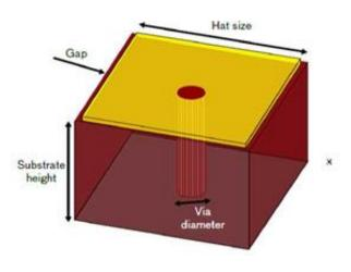
Figure 2. One unit cell Of AMC
