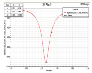
Figure 4. Simulated S11 response for conventional RMSA
