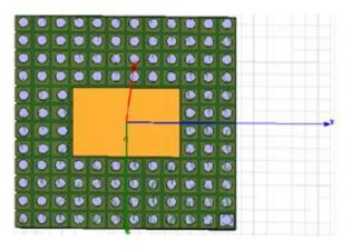
Figure 3. RMSA with AMC structure
