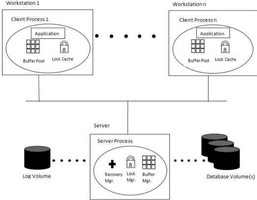
Figure 1. Client Server Architecture for proposed framework
