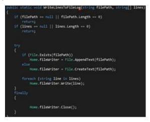
Figure 6. Method to write changes made by transaction to log
