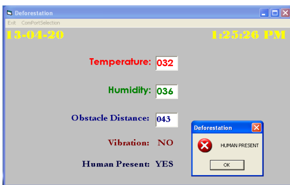
Figure. 6 Parameter Display in Control Station
