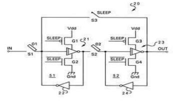
Fig 3: Multi-Threshold CMOS Technique
