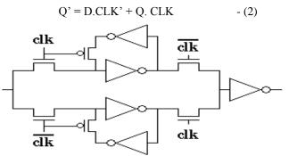
Fig 1 : Double Edge Triggering Flip-flop Equation (1) describes a latch which passes the input data when CLK= 1 and stores it when CLK = 0. Inversely, Equation (2) describes a latch which passes the input data
