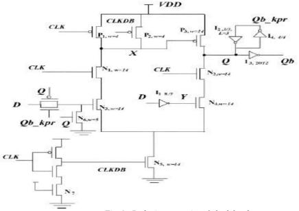
Fig 4 : Reducing capacity of clock load
