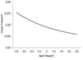
Fig 9: Output voltage of pseudo resistive divider
