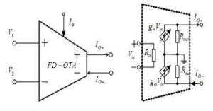
Fig 1: OTA (a) Symbol (b) Equivalent circuit
