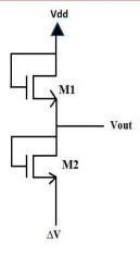
Fig 6 : Basic Pseudo Resistive Divider
