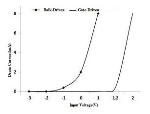
Fig 5: Characteristics plotted for Gate driven and Bulkdriven n channel MOSFET
