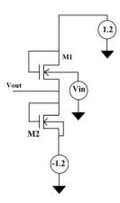
Fig 7: Pseudo Resistive Divider used for design
