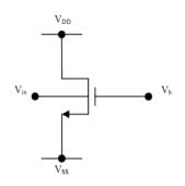
Fig 4: Bulk-driven MOSFET symbol
