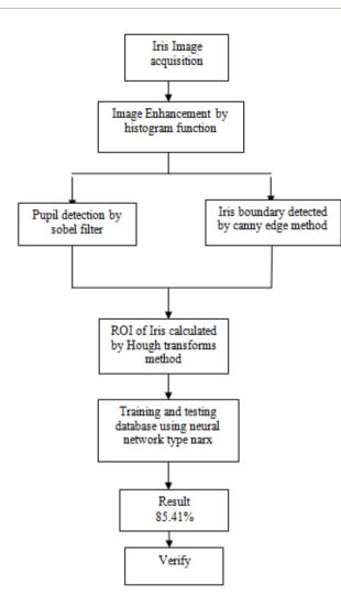
Figure 1. Flow chart of Iris recognition system
